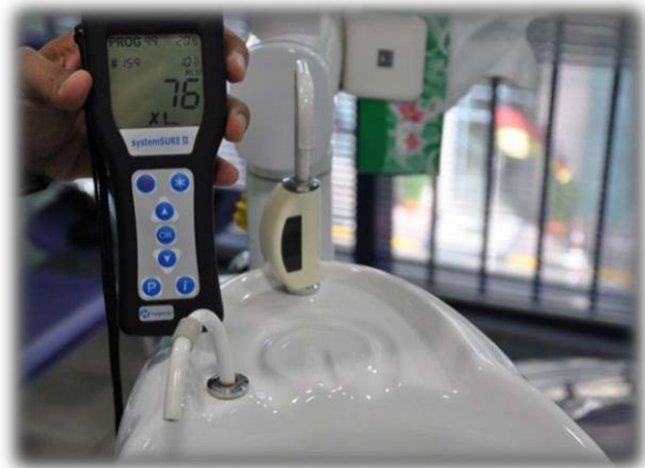
Spitting pool @ 76-dangerous
